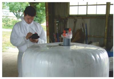
Detection device in a shock-resistant, dust-and-moisture-proof container registers gamma radiation of controlled radionuclides. Detection device sends spectrometric data to hand-held PC (Tablet PC) by wireless communication channel for displaying on screen.
