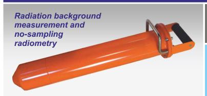
Multifunction portable spectrometer is designed for radiation control of water, agricultural products, seafood, raw materials and other substances without prior sampling and sample preparation.
